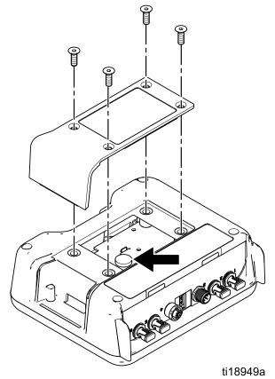
5. Use a flathead screwdriver to pry out the old battery.
